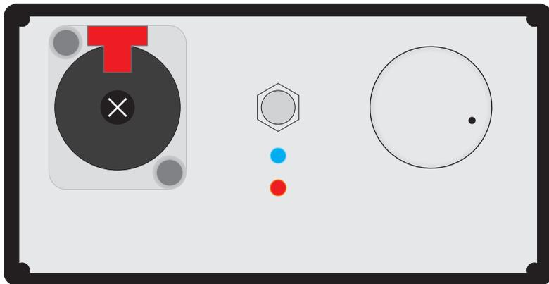
PPA + battery board, both LEDs showing, bass boost switch.
