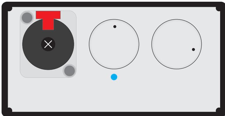
PPA + battery board, power LED showing, rotary crossfeed switch.
